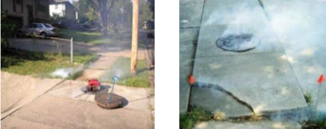
Figure 2. capacity blowers are used to pump non-toxic smoke into a manhole (left photo). In the right photo, smoke is pushed into the system and emerges from cracks in the sidewalk and at a downstream manhole.
